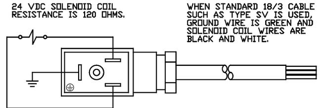
In some cases, the power source for the Compact Electric Valve actuation will be supplied internally from the pattern control/timer unit, so that the user will need only to supply a DC signal or passive contacts to activate the applicator.
